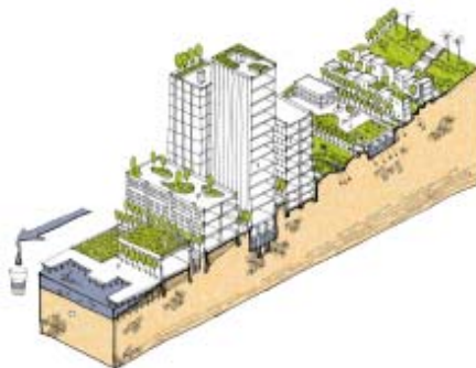
Impact of rising tides on San Francisco's combined sewer system (lt) Proposed low impact design to attenuate over taxed storm sewers includes: intensive eco-roof, rain screen, permeable paving, cistern, in-street planter (ctr) San Francisco Bay area's Wastewater System (rt)
