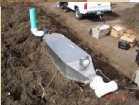
Dilution tunnel on windrow
