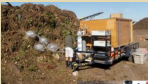
Flux chambers on tipping pile
